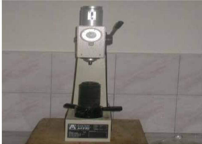
Gambar 3.4. Hardness Testers
