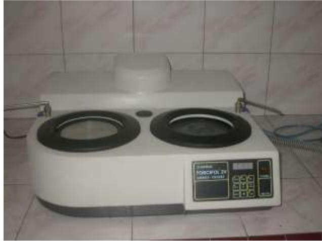
Gambar 2.1. Metallographic polishing table
